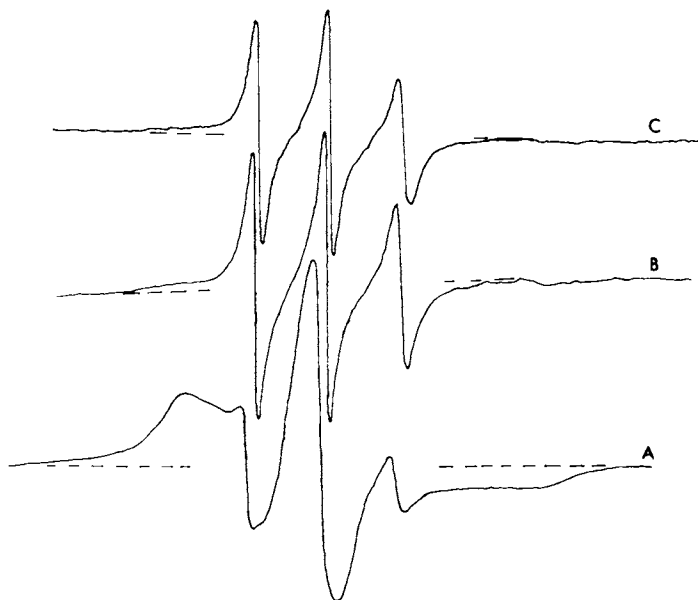
Figure 7. The dependence of the ESR spectra on surface coverage of PVAc (61,000) at the \text{SiO}_2(\text{Cab-O-Sil})\text{-CCl}_4 interface at 25^\circ\text{C} . Percent of saturation uptake: (A) 50%; (B) 90%; (C) at saturation.
